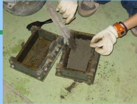
Steel moulds for fabrication of blocks
